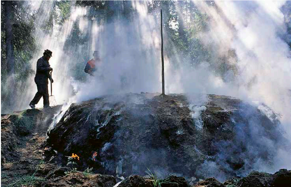
A tar kiln burns in the Seitsemien National Park. Tar has been used for centuries to protect boats and buildings. Tar became Finland’s most important export product for around a century after 1770. Around 30 litres of tar can be obtained from a cubic metre of pine wood.
