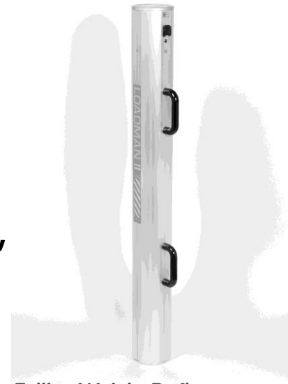
Loadman Portable Falling Weight Deflectometer
