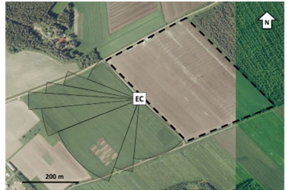
Fig. 1. Field site with the sectors representing the target area. Black solid lines indicate the borders of the sectors used in the footprint analysis of the EC flux data. The EC tower is located in the middle of the grass field, beside the road. The field surrounded by black dashed line is the north-eastern field, which had the same treatment as the study field during the campaign but a deeper peat layer.
